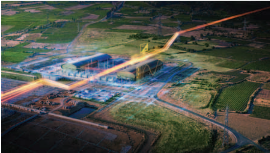
Converter stations at the ends of HVDC transmission lines invert and rectify the current flow by converting AC to DC and vice versa
